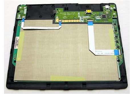
Interior view of a Wacom tablet
